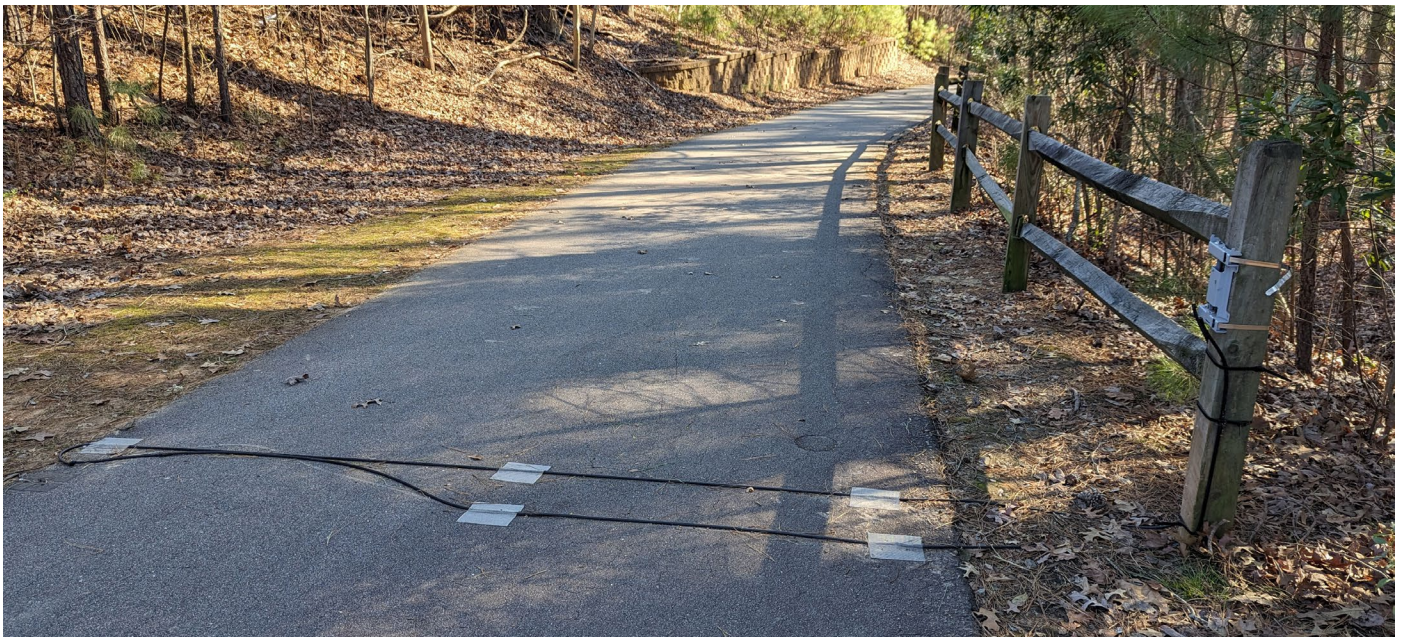
A trail counter device on the Black Creek Greenway in Cary, NC collects data about greenway usage.
