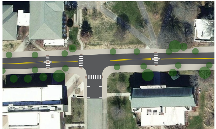
Narrow sidewalks and wide roadway lanes increase the crossing distance for pedestrians on this busy corridor.
