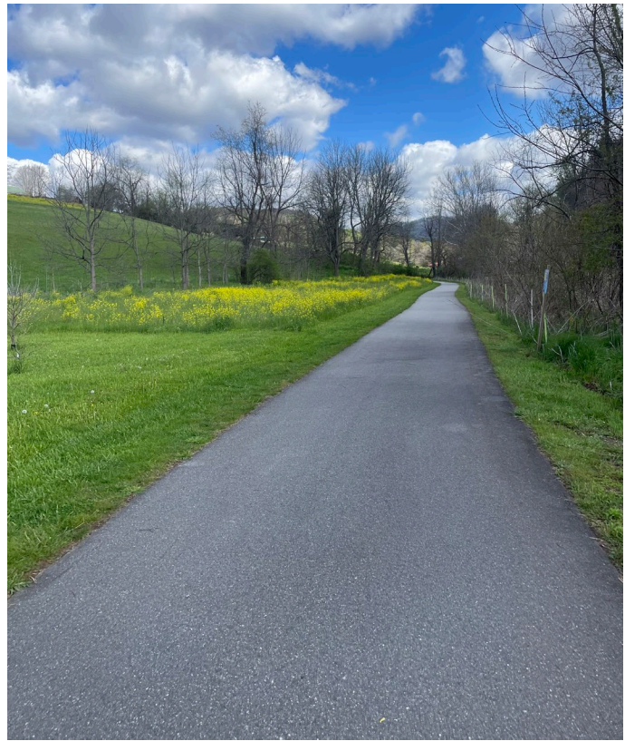
The Dr. W. Otis Duck Memorial Greenway has an asphalt paved surface with a 10 ft width in most locations.
