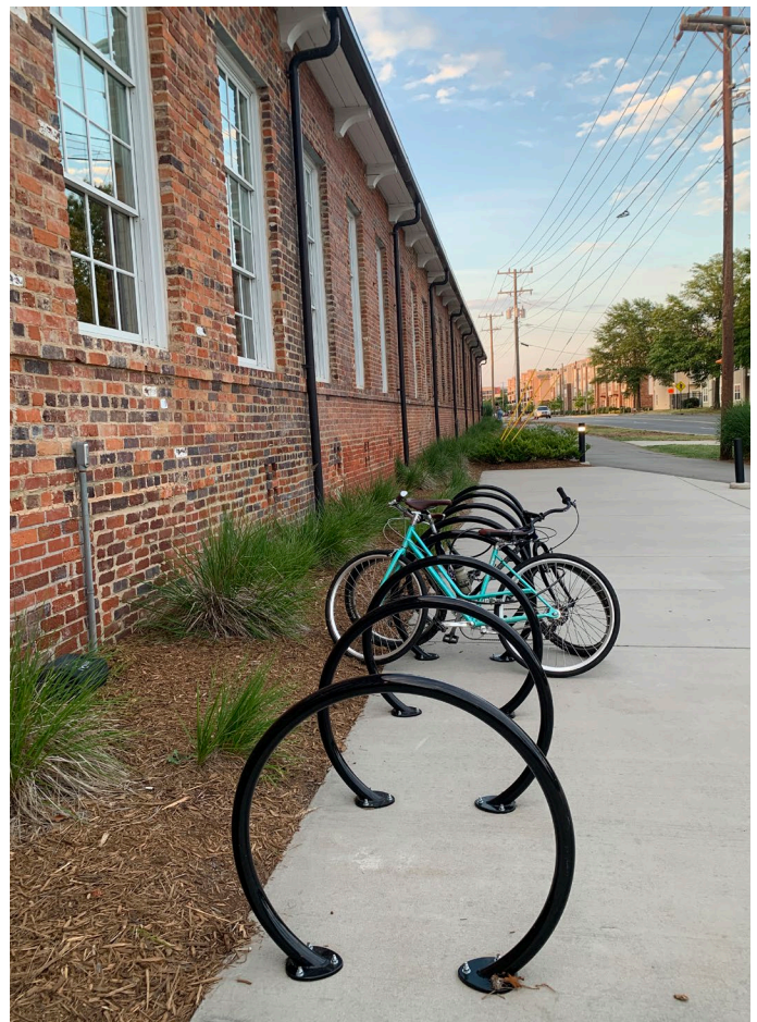
A good bike rack provides two points of contact between the rack and the bicycle, as seen at this bike rack in Charlotte, NC.
