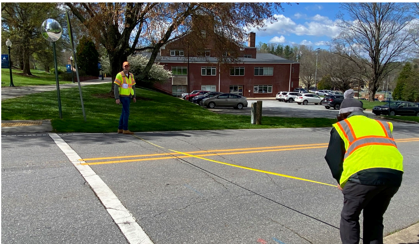
Roadway width is a factor in the selection of bicycle and pedestrian facilities and crossing treatments.
